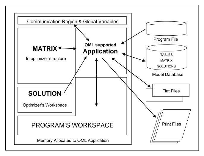
OML provides access to and control of the entire model environment.
